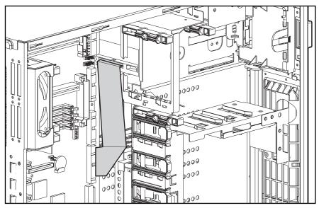
Figure 2-24. CD-ROM drive cable folding and routing diagram
